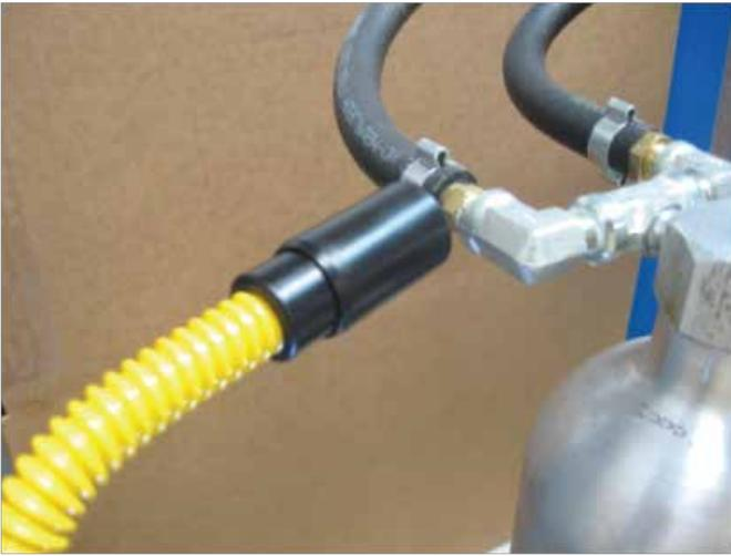
**Step 15.** Using the electronic leak detector go around the system to identify the leak site area. While moving the CO2 probe tip around the system it is best to keep the CO2 sensor face perpendicular to the surface being tested. **Note: If tip is bumped against the surface being tested the detector may momentarily go off, this false alert will go off right away. If the leak detector senses CO2 gas the alert will stay on for 10 to 40 seconds.**
