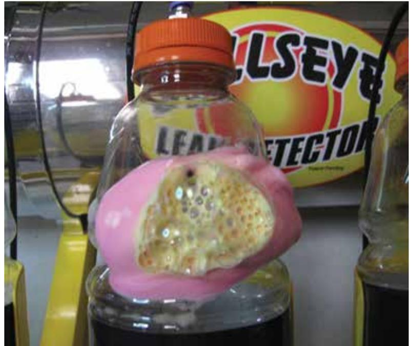
**Step 19.** On large leak sites the Bullseye Leak Seeker Solution will bubble and change color from pinkish red to yellow indicating a larger leak site.
