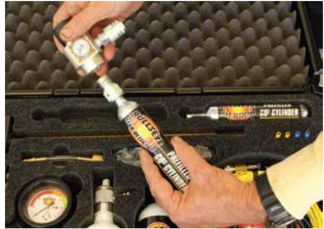
**Step 21.** Unscrew the high pressure regulator from the 90 gram CO2 cartridge and adaptor.
