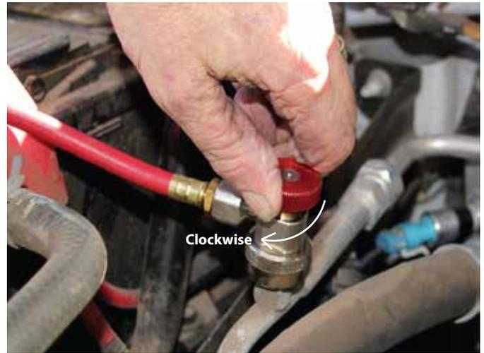
**Step 12.** Now rotate the Bullseye High Side R-134A Adapter knob clockwise this will open the valve and will allow CO2 to flow into the vehicles air conditioning system thus pressurizing the system.
