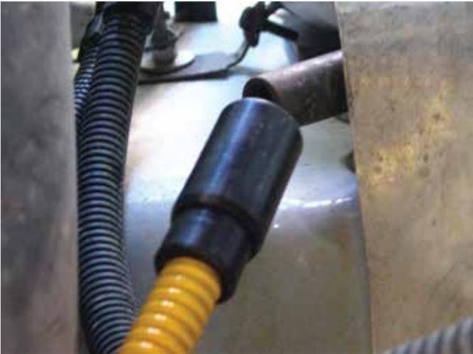
**Step 20.** If no leak is found place CO2 detector at EVAP drain hose and remove cap plug while leak detector sensor is near hose outlet. CO2 is heavier than air and will fall to the bottom of the EVAP housing accumulating in the drain hose. If the Bullseye Leak Detector detects CO2 at the EVAP drain hose there is a leak present somewhere in EVAP housing. Note: For best results leave the system under pressure for 30-60 minutes **or longer** before removing cap plug from drain hose.
