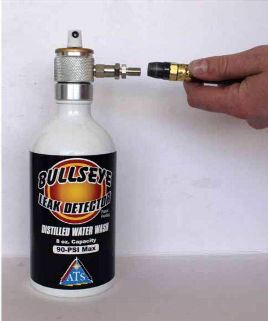
1. Depress schrader valve and release any air pressure remaining in bottle.
