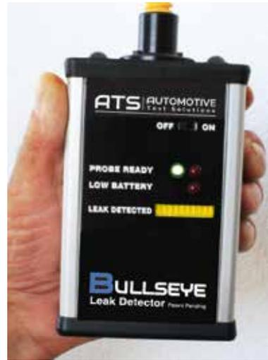
**Step 6.** Remove electronic leak detector from kit and turn on the unit, allow unit to warm up the CO2 sensor tip. When unit is ready the red light will shut off and the green ready light will turn on, this will take about 90 seconds. For best results the leak detector CO2 sensor should be allowed to fully warm up for about 5 minutes.
