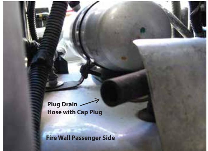
**Step 14.** The EVAP housing will have a drain hose to drain the moisture from the EVAP core. This hose is usually located on the passenger side lower fire wall in the engine compartment. Plug this drain hose with a cap plug from the Bullseye kit while the rest of the system is tested for leakage.
