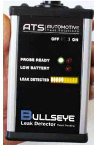
**Step 16.** When CO2 gas is detected the LED display bar is activated along with the audio alert (loud beeping noise). Once the detector has sensed CO2 the alerts will continue for about 10 to 40 seconds; **Note: Remove sensor from leak site area and let the unit stop beeping on its own.** Once the detector has stopped beeping you can now retest the leak site area with the CO2 detector.
