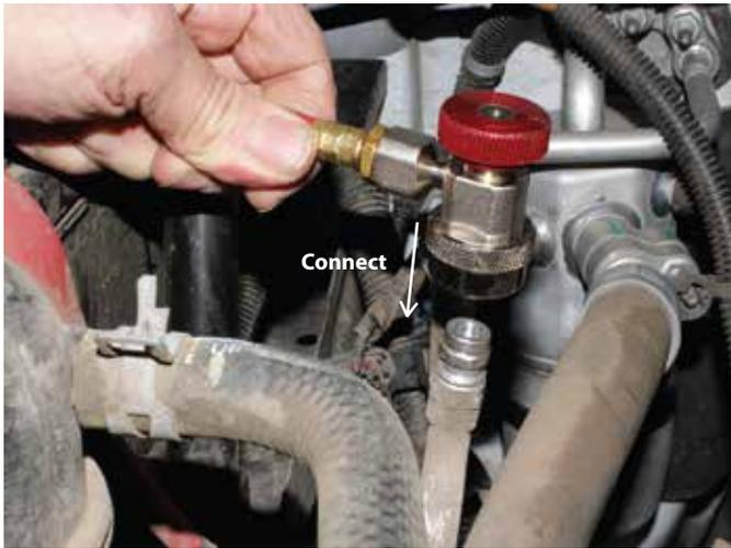
**Step 11.** Connect the Bullseye High Side R-134A Adapter to the vehicles high side charge port.
