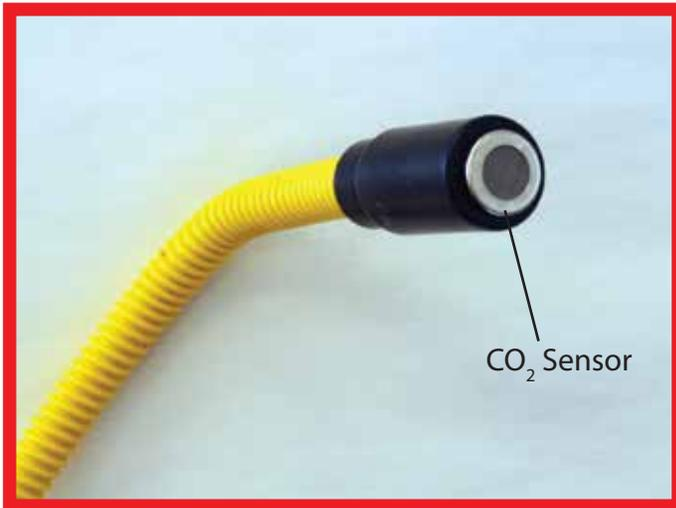
**WARNING!** Do not allow leak seeker foam to get on CO2 sensor at end of yellow flex tube! This will damage CO2 sensor and will require the CO2 sensor to be replaced.
