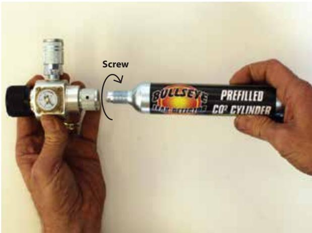
**Step 7.** Remove high pressure regulator with adaptor from kit and screw CO2 cylinder to high pressure regulator.
