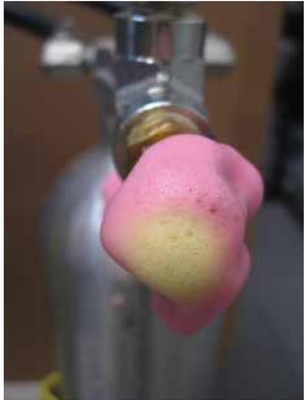
**Step 18.** The Bullseye Leak Seeker Solution will spray on pinkish red and turn yellow at the leak site. On very small leak sites no bubbles will form. This is due to a very low gas volume escaping from the leak site.
