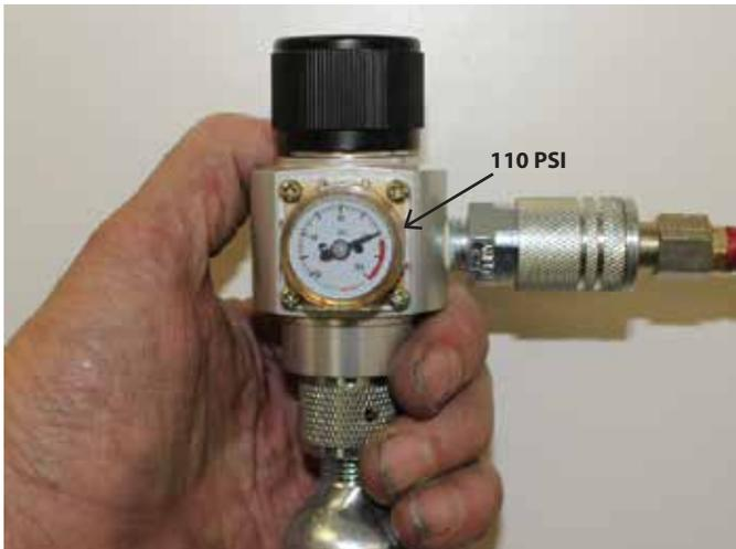
**Step 13.** Watch the high pressure gauge on the front of the high pressure regulator; make sure it stays greater than 110 PSI. If a large leak is present you will not be able to pressurize the system to 110 PSI. In this case you will need to repair the large leak and then retest the system. If the pressure gets to 110 PSI and then drops you may need another CO2 cartridge in order to maintain the 110 psi level.
