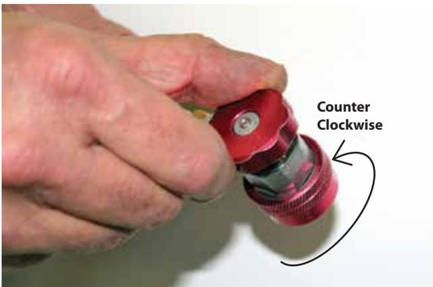
**Step 9.** Close the valve on the Bullseye High Side R-134A Adapter coupler by rotating the knob counter clockwise. Bullseye Adapter may not be included in your kit. (Order ATS part # LDT1350.)
