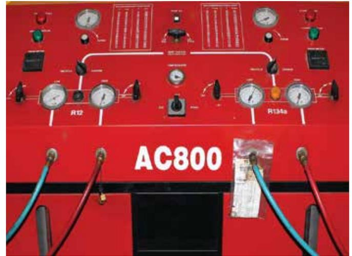
**Step 2.** Recover all the refrigerant followed by a system evacuation that will help maintain a vacuum in the condition system.
